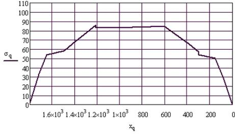
FIGURE 8. Maximum bending stress,  $N/mm^2$
