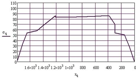
FIGURE 12. Maximum bending stress,  $N/mm^2$
