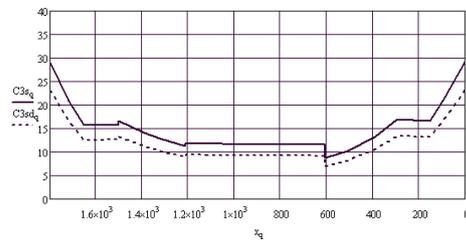
FIGURE 19. Safety coefficient in simple bending; as to  $C_{sdq}$  flow limit; as to  $C_{sq}$  resistance to breaking
