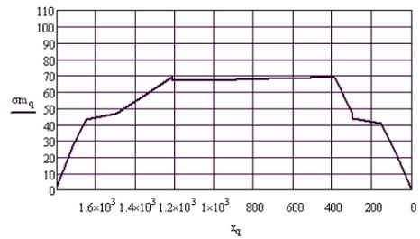
FIGURE 13. Minimum bending stress,  $N/mm^2$
