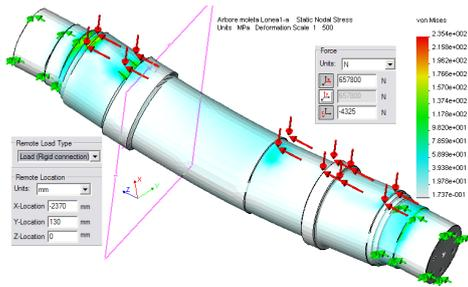
FIGURE 21. The pulley shaft stressed in the wedge canal on its opposite face on the level on the bearing sidet
