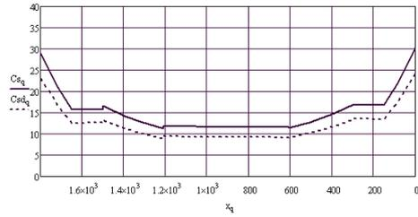
FIGURE 11. Safety coefficient in simple bending; as to  $C_{sdq}$  flow limit; as to  $C_{sq}$  resistance to breaking
