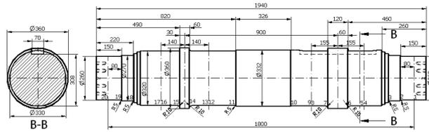
FIGURE 5. Constructive size of the shaft
