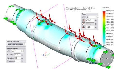
FIGURE 22. The pulley shaft stressed in the wedge canal plane on it opposite side on the inside level
