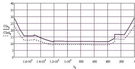
FIGURE 15. Safety coefficient in simple bending; as to  $C_{sdq}$  flow limit; as to  $C_{sq}$  resistance to breaking
