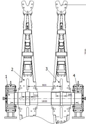
FIGURE 4. The pulley shaft
